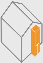
The elevator is built on site in **a lift shaft by the assembly team.** The shaft can be erected on the exterior or as additional building, depending interior of the house.
